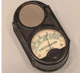
Fig 7. Weston Model E703 Lightometer for measuring general light intensity (Taranovich 2016)
