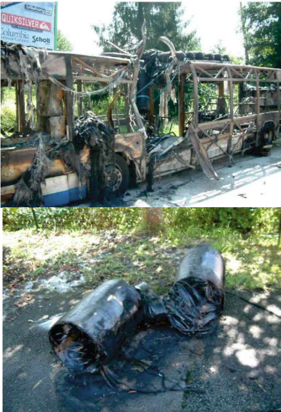
Fig.27.: The burned out bus in Montbéliard, and the residue of the cylinder, which splitted in two parts. The initial problem came from the electrical circle of the bus [24]
