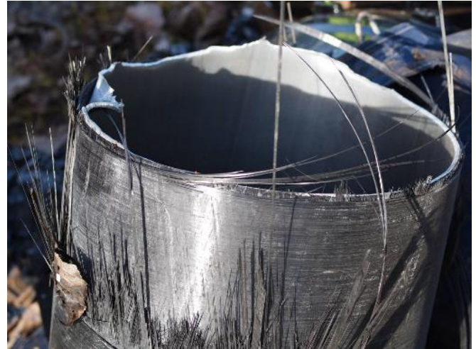
Fig.30.: The carbon fibre wrapping was capitulating way under the design pressure. In the middle, the metal liner material flown. [Author]
