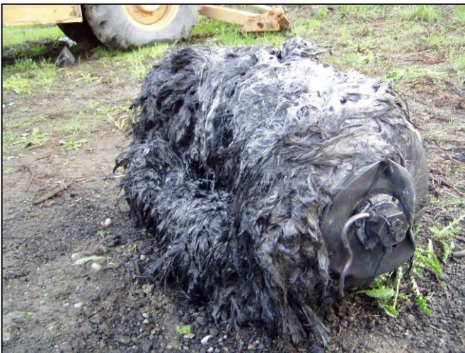
Fig.25.: The bursted and burned cylinder residuum from the Civic [27]
