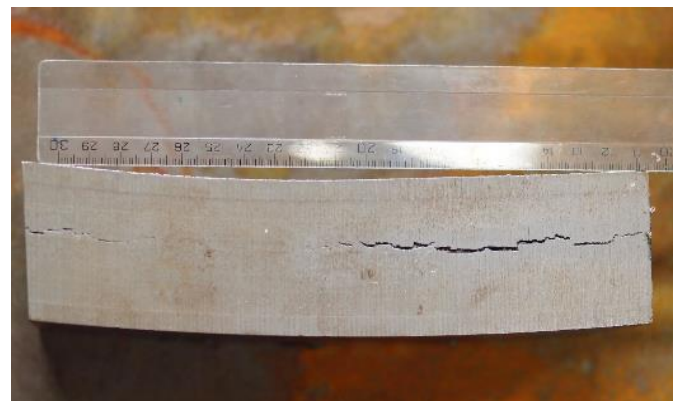
Fig.4.: This excised piece of a hydrogen industrial spherical container shows the hydrogen accumulation deep in the 50 mm wide steel plate, which was even able to straighten the inner side. Under heat and pressure the Hydrogen bubble created bursting force is over 100 MPa range. [Author]
