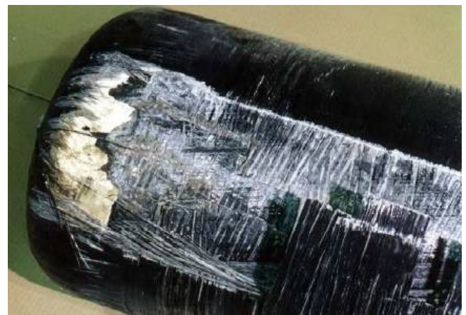
Fig.23.: Bus tank after impacted with an over-bridge [28] Cannot miss from this list, the cylinder's improper treatments, like an event as falling. That can occur an external abrasion, or damaging on the surface of the wrapping by sharp, abrasive tools and through effecting the fibre-epoxy structure.
