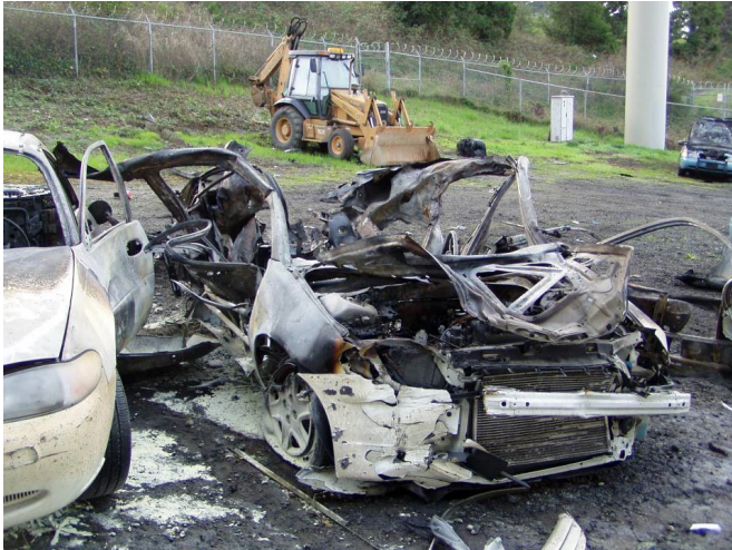
Fig.24.: The case of a CNG propelled Civic in 2007 in Seattle, where the PRD was not opening and actuating releasing the gas. The ruptured tank was landed beside of the excavator [Photo 23, 27]
