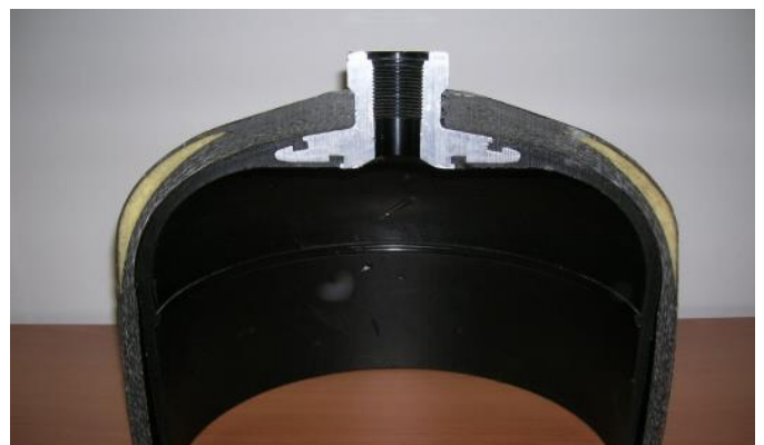
Fig.13.: Type 4 vessel cross section at the neck part
