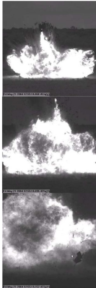
Fig.28.: Fireball captured by IR camera, from above, 10 msec, 45 msec, 107 msec after the rupture [25]
