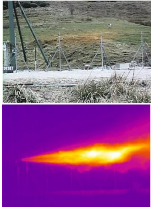
Fig.2.: Comparison between the visible flame (above) and the flame extent obtained through thermal imaging (under) (Moonis et al., 2010, taken from [8])
