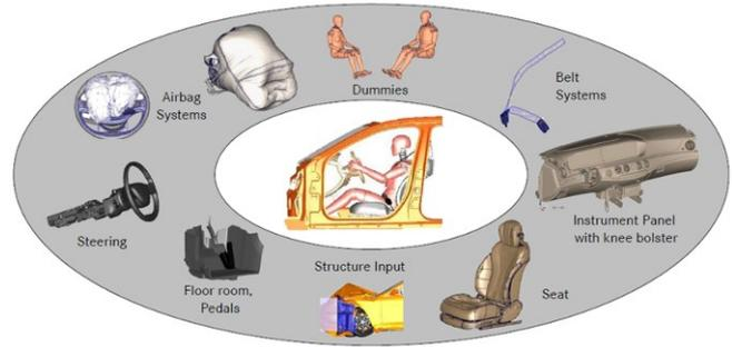
Fig. 4. Occupant safety simulation components
