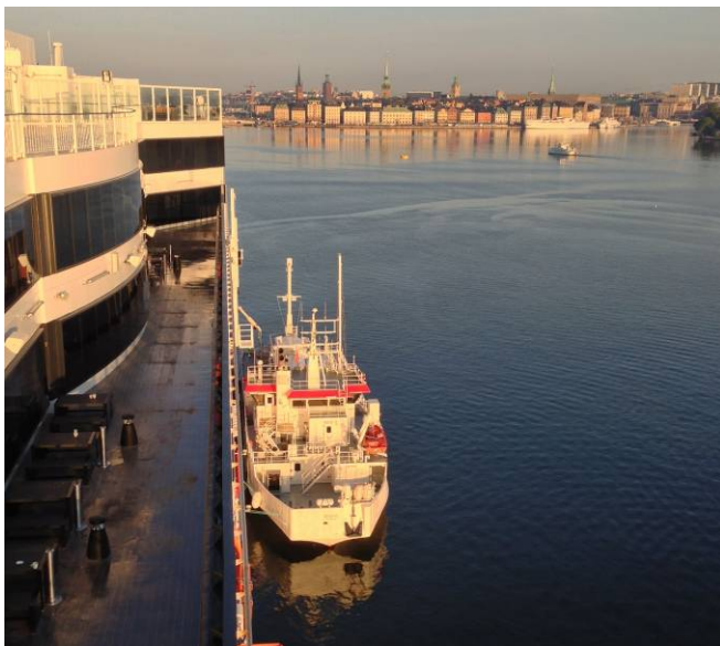
Fig. 4-13: The world first hybrid-gas powered Ro-Ro ship Viking Grace is being refuelled by the tailored bunker ship in Stockholm. The process is monitored from the bridge through computer as well via video stream [image: Author]
