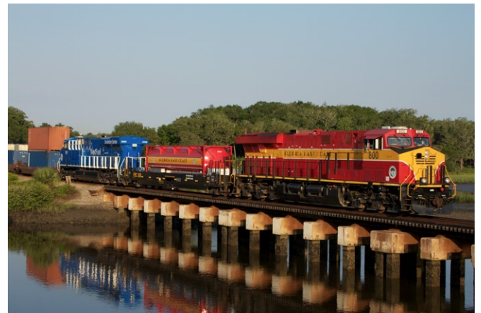
Fig. 4-4: Beside of others Florida East Coast Railway employs LNG powered locomotives. It shows not only highly remunerative figures, but clean air and far lower engine noise level is also proved [image: Michael Maiullari/Trains Magazine]
