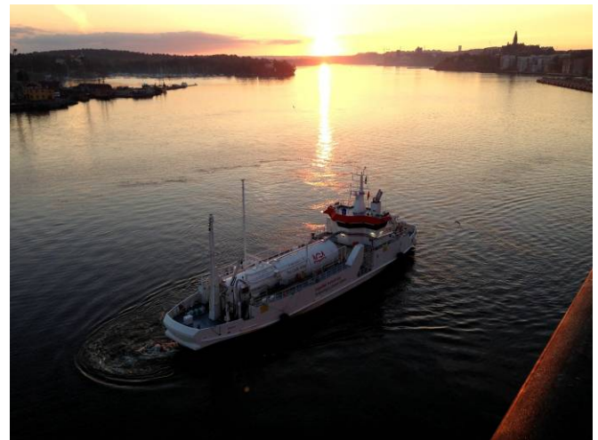
Fig. 4-11: A retrofit bunkering ship by AGA, fuelling the hybrid-LNG powered Viking Grace Ro-Ro ship in Stockholm every morning. The Viking Grace has approximately 50 t daily consumption, while 150 t storage tank on-board. The refuelling takes less than an hour, including connecting [image: Author]
