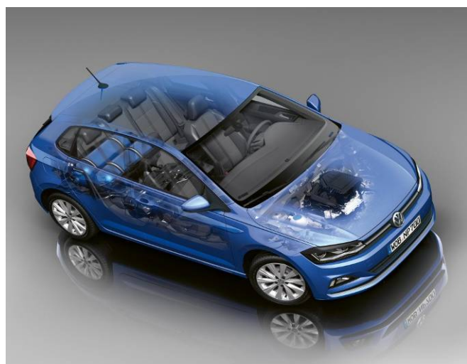
Fig. 4-2: Volkswagen Polo TGI, equipped with a modern 1,0 litre turbo spark ignited engine, optimized for CNG [image: Volkswagen]
