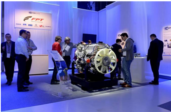
Fig. 4-3: display of a next coming gas engine technology from FPT on the HDGAS Project closure event. The direct injected, crown-type ignited engine, variable valve timing engine runs in test benches with stoichiometric as well lean-burn principle and produce 2200 Nm, 370 kW beside of 14 % reduction in GHG, compare to the existing one [image: HDGAS Project]. Direct gas injection, as well pre-chamber solutions are coming, latest bench test results are demonstrating at small 1-1,5 liter engine category, that 44 % peak efficiency is possible, which goes above today's diesel values
