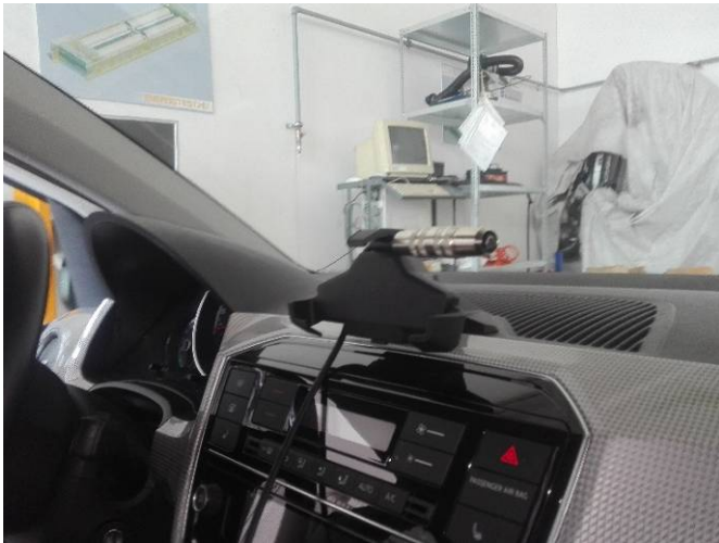
Figure 4: Measure set up (microphone in the passenger compartment)
