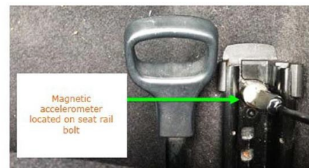
Figure 3.: Measure set up (OBD and Accelerometer)
