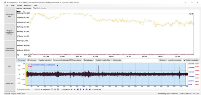
Figure 6: Pikes indicates the A/C compressor
