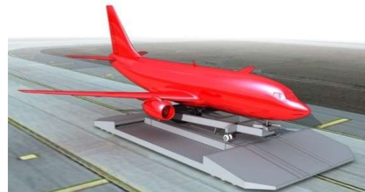
An example of the investigated emergency landing solutions: lightweight skids (left) and emergency cart (right).
