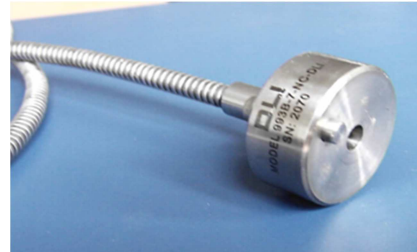
Figure 3. A triaxial vibration sensor commonly used in condition observing systems – manufactured by Wilcoxon (USA).
